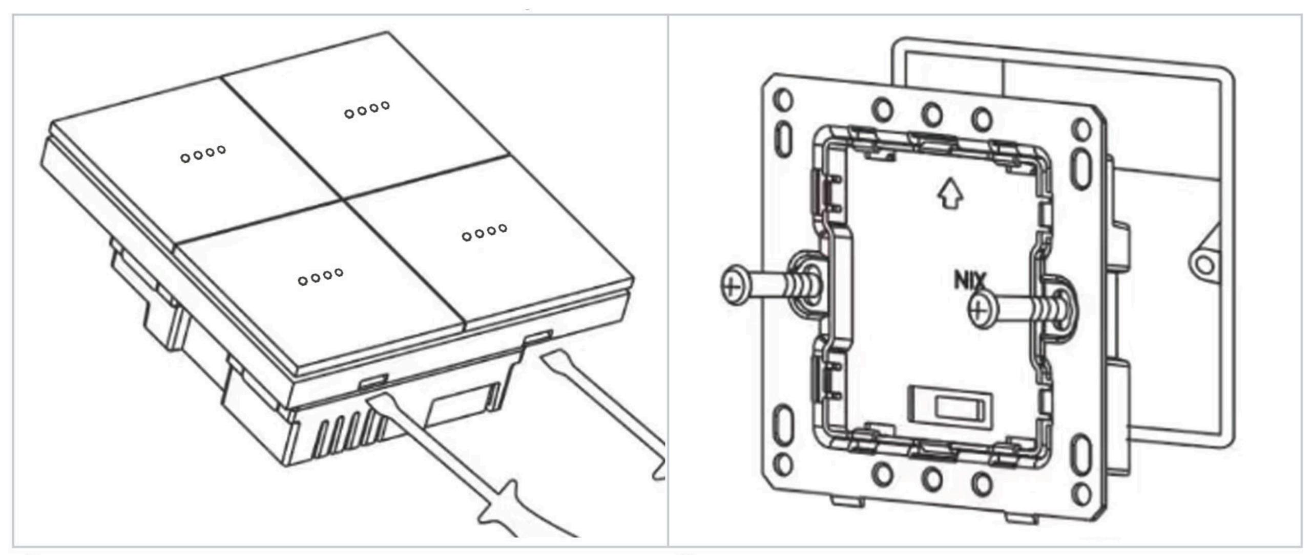
1) Use a screwdriver to pry the panel upwards;
